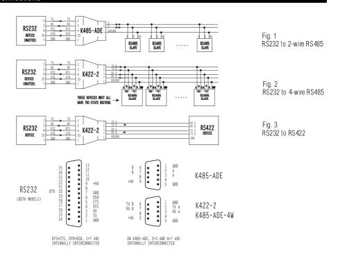
The K485-ADE is intended to plug directly into a standard 25-way IBM PC RS232 port. If your PC has a 9-way RS232 port, you will need the commonly available 9-25 moulded converter. Alternatively, the K422-99 and K485-99 products (without ADE) are available for 9-way ports.
