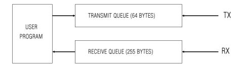
A user program never accesses a port *directly*; any **READ**, **WRITE** etc statements communicate only with the queues. The transfer of data between a queue and its port is performed as a background process (i.e. under interrupts) by the comms processor and is transparent to the user program.
