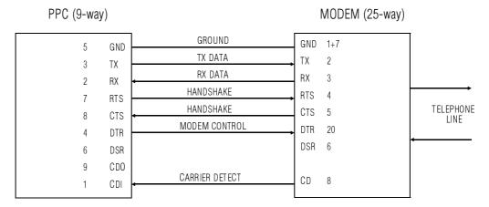
The PPC port should be configured with the following handshakes:
