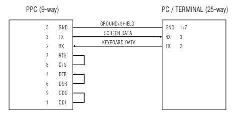
This cable is designed for use with the KTERM.EXE terminal emulation program. Some terminals and terminal programs (e.g. PROCOMM) require a high level on their CTS and/or DSR inputs (pins 5 & 6) before transmitting data; this can be most easily achieved by interconnecting RTS+CTS+DSR (pins 4+5+6) on the terminal.
