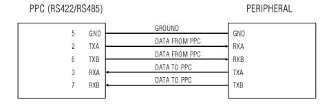
In a multidrop system, with the PPC acting as the Master, there can be multiple peripherals (Slaves). All the Slaves have their connections parallelled.
