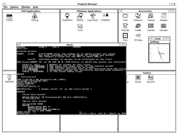
Note that KTERM will initially be invoked in the basic mode with no command line options, at 9600 baud. You may wish to edit the command line (in the KTERM.PIF file or in the Program Manager Properties menu; see your Windows Manual) to select e.g. a 50-line VGA mode (/VL option) and a higher baud rate. The above screen shows KTERM running with the /VL option under Windows 3.0 with a super-VGA (1024x768) display in 386 enhanced mode.
