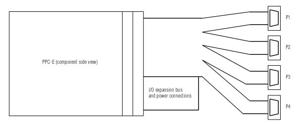
With the above cable arrangement, the pin connections of the DB9 connectors are identical to those of the standard PPC-4 product.
