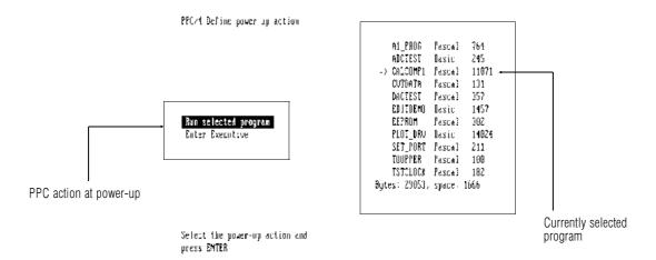
You can instruct the PPC to either automatically compile+run ("autoexec") the selected program, or to always enter the Executive. The selection is stored in non-volatile memory.
