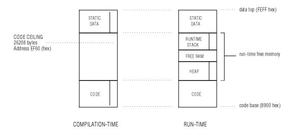
Static data is allocated during compilation from top down, and can extend *almost* all the way down to top of code. What is left in between will be the *run-time free memory*, and the compiler will always leave at least 512 bytes spare. As an example, in a program which contains
