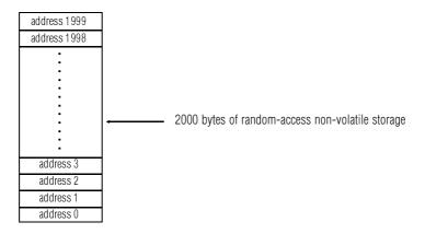
This is a very useful feature which permits the construction of a device which can self-modify its properties and retain the changes through power-down. Examples include the storage of passwords in a security device, or the storage of calibration coefficients for the analog subsystem.
