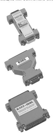
A range of high quality very low cost RS232 to RS422/485 converters is available. All units plug directly into an IBM PC serial port (25-way or 9-way) and are line-powered from the RS232 interface's RTS or DTR signals. Isolated models (1kV RMS test) are also available.
