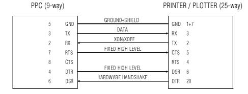
The un-named connections do not usually serve any purpose except to supply an RS-232 HIGH level to the device's CTS and DSR inputs. For example, some plotters will ignore incoming data, or (e.g. in case of HP pen plotters) will not respond to interrogation commands, unless those inputs are HIGH.
