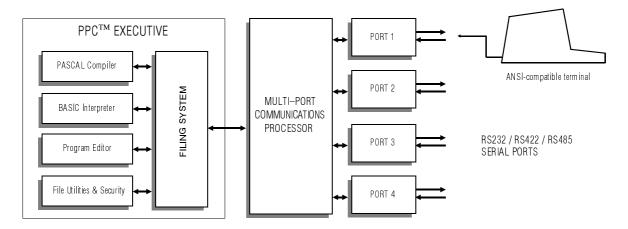
An ANSI-compatible "dumb" terminal is the only additional equipment that is required, and it can be disconnected once the program is finished. All PPC configuration is done via the terminal; there are no internal switches.
